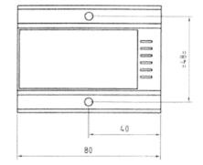
The device has been developped adjust the rotation speed of a direct current motor (or the light capacity of an electric bulb), by means of the regulation of the voltage. The adjusting range is between 0 and 100% of the rotation speed (or light capacity).
